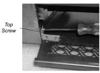
4) Attach the two control boxes to the bottom unit base and tighten the 2 screws on the left side and 1 screw on the right side.
